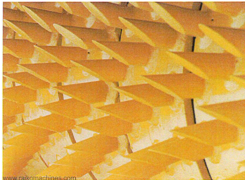
Freely rotating spiked roll system with high quality bearings and individual roll absorbers
